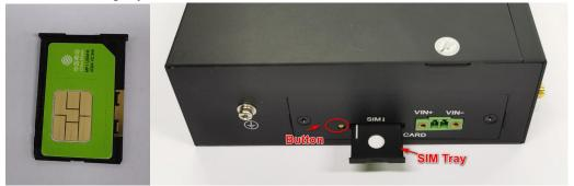
Warning: DON NOT install SIM/UIM card when router is powered on.
